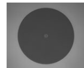
Click to Enlarge Undamaged Fiber End
